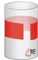
Fig. 10-4: Product with position displacement of the label
