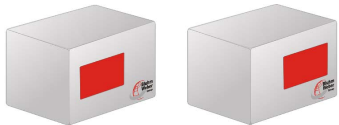
Fig. 10-4: Product with position displacement of the label
