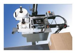
The Model 5300 Corner-Wrap system operates using Weber's Legitronic Labeling Software, which facilitates the formatting and printing of labels and also combines RFID encoding, if required.
