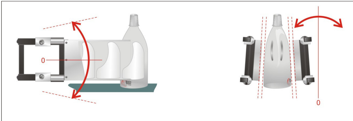
Fig. 7-13: Inclination angle of peeler plate with gimbal
