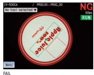
Detection of sticker presence/absence by using position adjustment
