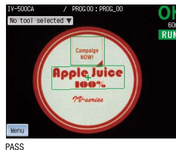
Detection of sticker presence/absence by using position adjustment
