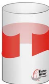
Fig. 7-7: Product with wrinkles in label
