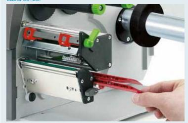
The label sensor can be unlocked with finger pressure and removed for cleaning.
