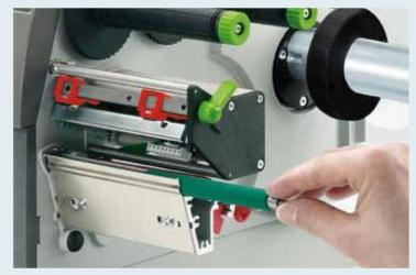
For cleaning or replacement, the print roller can be easily removed by loosening just three screws.
