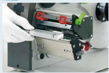
It takes only a few simple steps to exchange the printhead. Adjustments and settings are not necessary.
